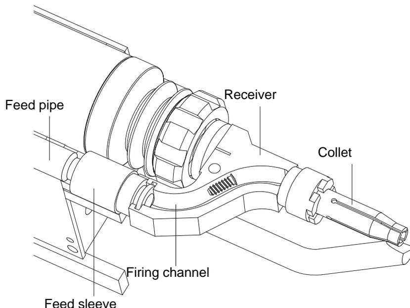
**Remark:** If no stud arrives in the collet, the loading and feeding times must be corrected. Afterwards repeat verification procedure.
