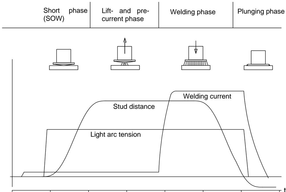
1. The required condition for the welding process is contact of the weld stud with the work surface (SOW), so that when the start command has been given the weld circuit will be electrically shorted via stud and work piece.
