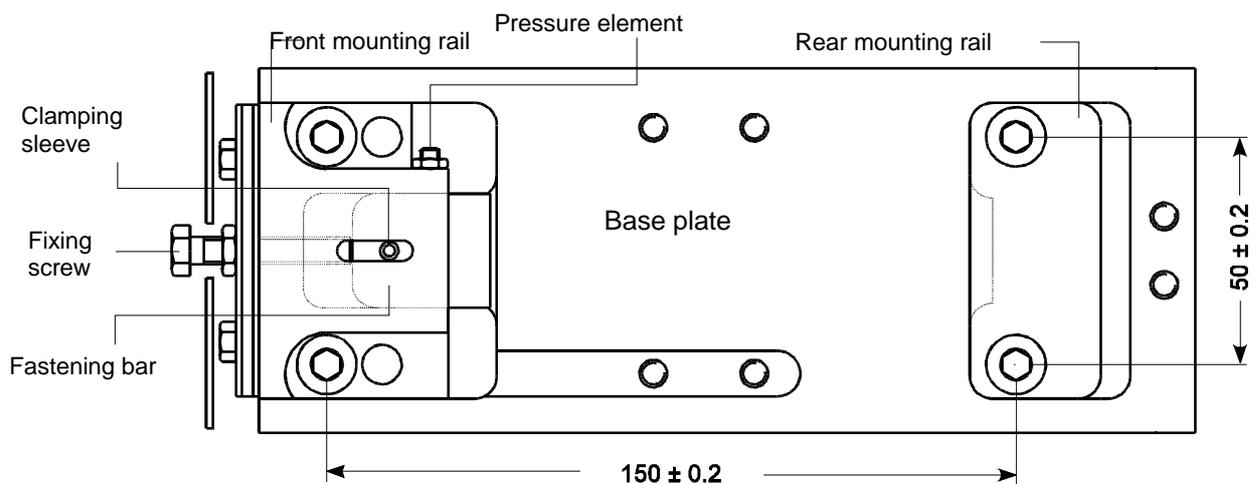
Having completed the assembly, verify smooth running of the weld head slide rail by moving it manually from the front end to the rear end of travel.
