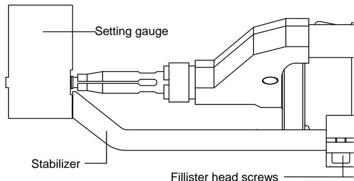
If stabilizer and stud are not on one level (when welding edges), the plunge depth can not be adjusted via the gauge. In this case the plunge depth is to be established empirically.
