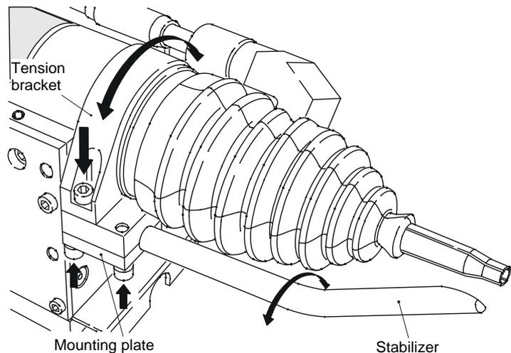
5. To achieve this, release one of the two M6 fillister head screws of the tension bracket and rotate the tension bracket together with the stabilizer around the longitudinal axis of the weld head.
